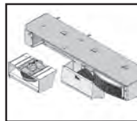
Figure 10. Cassette Removal (Step 5)
