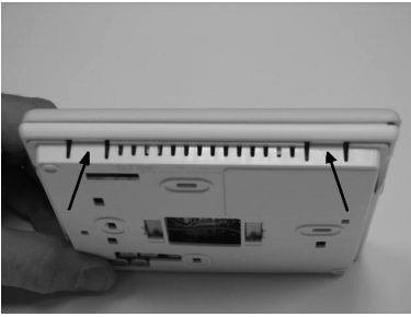
Fig. 5 - Press Tabs to Remove Backplate
